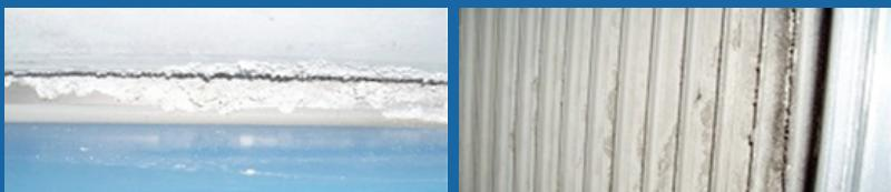
6 weeks later calcium deposits in the washing chamber were completely removed.
