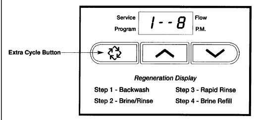
A. Once the valve reaches Regen Step #1 let water run to drain for about 5 minutes.
