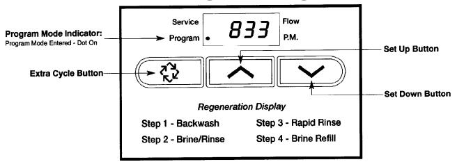
The first option setting display that appears in the Program Mode is Treated Water Capacity. Using the Set Up or Down Buttons, set the amount of treated water that can flow through the unit before a regeneration is required. For Example:
