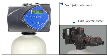
The residential 7000XTR offers a two-line, sixteen character LCD backlit display for easy entering of master, diagnostic, and user programming. No need to memorize codes or letters to program or read screens! Time of day is maintained during power failures, offering peace of mind and steady, treated water as needed.
